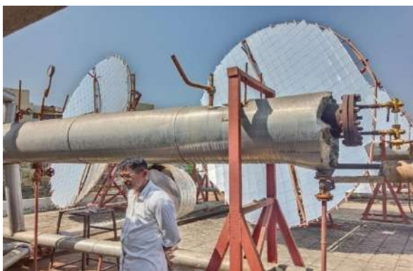
Parabolic Solar Concentrator
